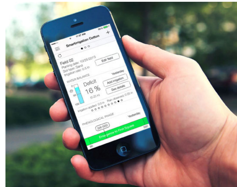
Figure 1. Screenshot of the SmartIrrigation Cotton App indicating how users can view data from multiple fields or zones as well as from up to nine previous days. The root zone soil water deficit is displayed both graphically and numerically in the center of the screen.
