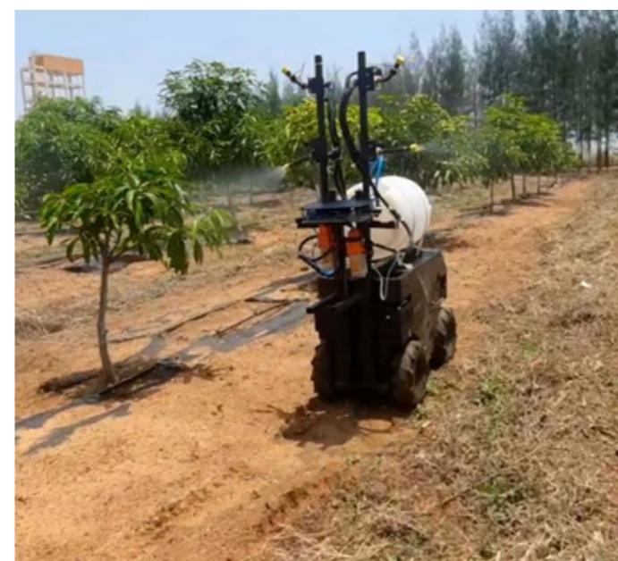
Pesticide Spraying with X100 Robot during farmer's field demonstration
