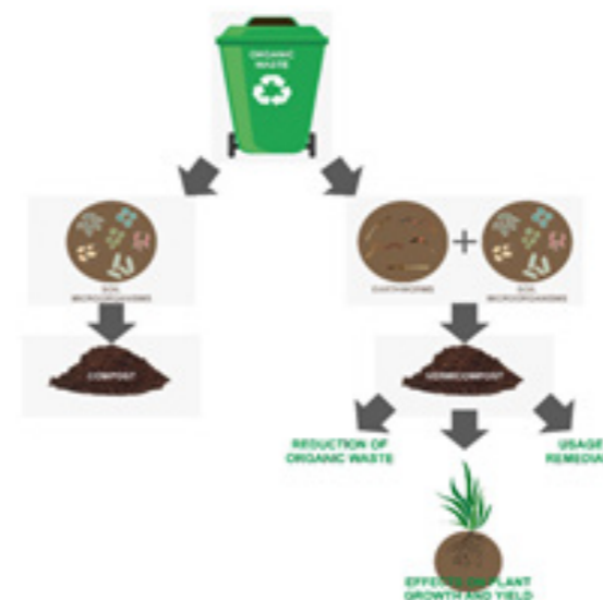
Fig.1. Conversion of organic waste into compost and vermicompost and the potential uses of vermicompost
