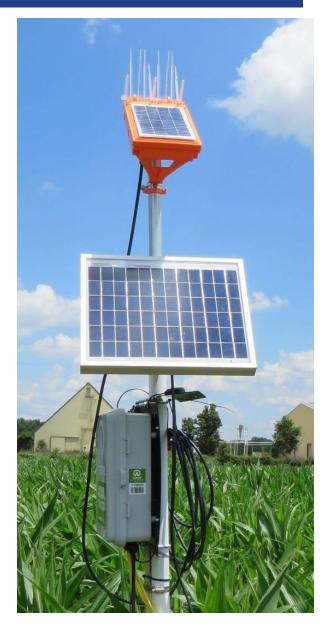
(FDR)- It is based on the principle that circuit frequency changes with changes in dielectric constant of the soil. It sends electromagnetic signal with the help of an oscillator through a wave guide or metal tine. Example-EC-5 and 10-H. In most cases it gives continuous changes in moisture level thus helpful to schedule irrigation as and when required.
