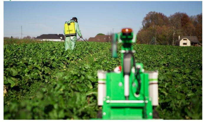
French company, Naio Technologies' Oz agribot, removes weeds and is designed to improve working conditions and reduce daily workload. It is an entirely autonomous agribot, but it can be guided and controlled to wherever it is needed. Oz needs to be informed of how many rows it needs to weed, the length of the rows and how far they are apart. When Oz has completed its weeding tasks, the operator will receive a text message directly to their smartphone.
