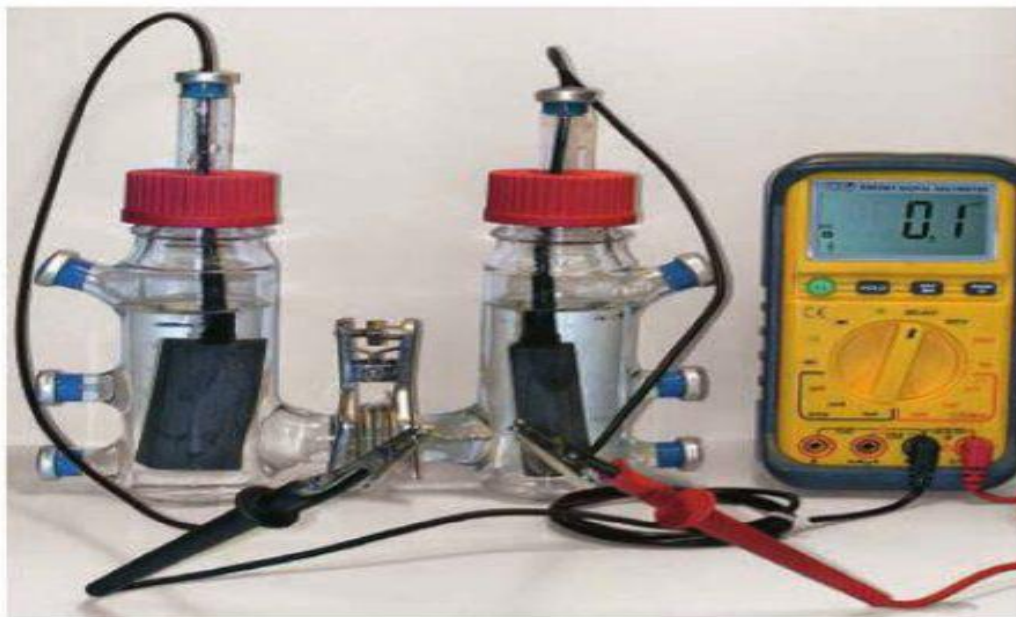
Fig 1: Two chambered microbial fuel cell
