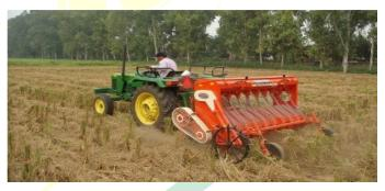
Adjust the depth of sowing through depth control wheels instead of using the hydraulic lift. Using the hydraulic lift to control the sowing depth may cause the touching of flails to the ground which may damage flails and also cause uprooting of the anchored residue. The ground clearance of the flails must be about 2.5 to 3 cm broken flail must be replaced before the further operation of the machine.
