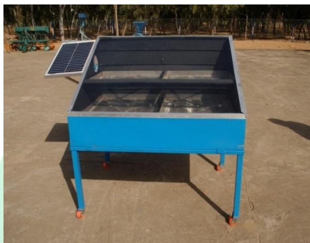
Fig. 4. PVT hybrid solar dryer installed at CAZRI solar yard
