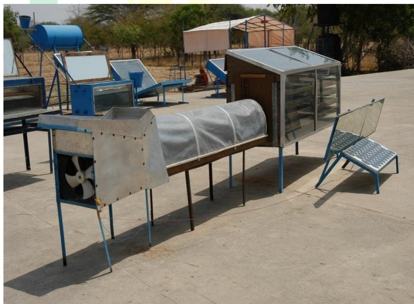
Fig. 2. PV winnower cum solar dryer
