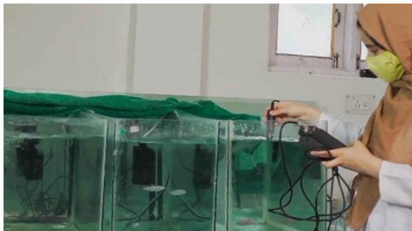
Figure 1: Checking water quality parameters in an aquarium set-up for trout fingerlings at Experiential Unit, College of Fisheries, SKUAST-Kashmir
