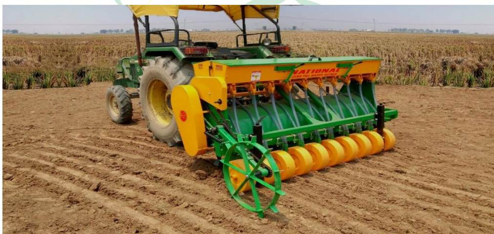
Figure: A Happy seeder operated for stubble management
