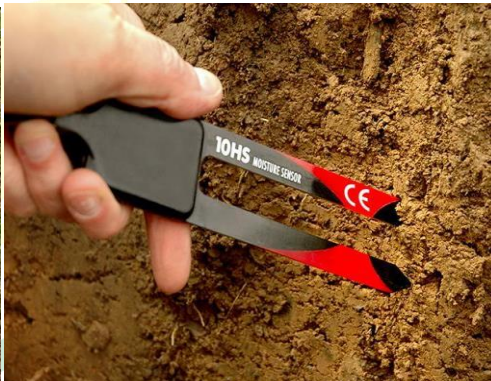
Fig. 2: FDR (Frequency Domain Reflectometry)
