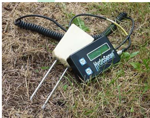
Fig. 1: TDR (Time Domain Reflectometry)
