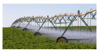
mounted on wheeled towers with a central water supply and a network of pipes and sprinkle's extending radially. When the center pivot moves around the field, water is sprayed evenly, providing crops with uniform distribution with controlled water supply in a continuous manner.
