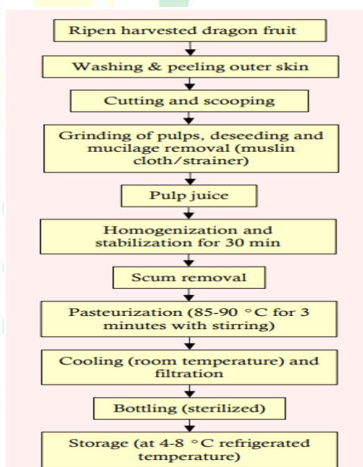
Fig.5. Dragon fruit juice preparation process flow chart
