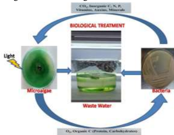
Fig.1. Symbiosis interaction between microalgal and bacteria in the wastewater treatment
