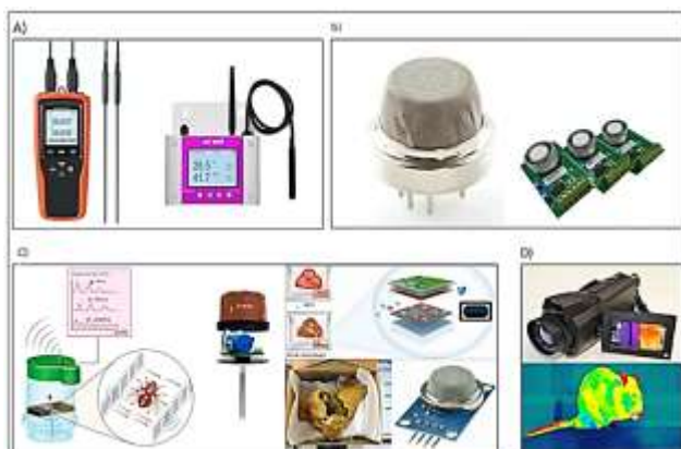
Figure 5: a) Temperature and humidity sensors b) Gas sensors, insect and fungal detectors and d) Rodent detectors (infrared cameras) (Source: Ahmed et al., 2023)
