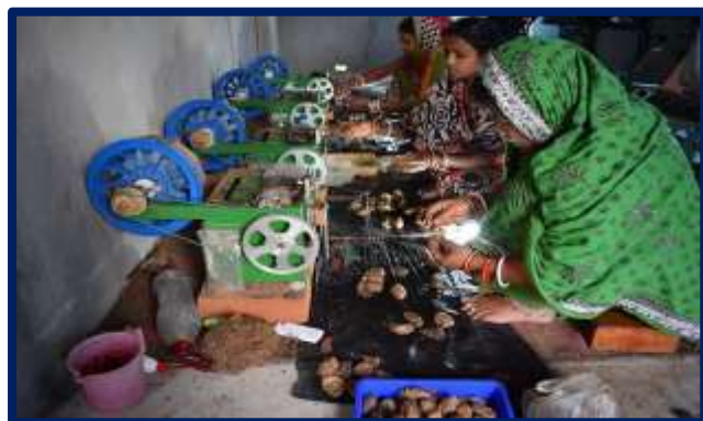
Figure 1. Traditional Charkha reeling machine used for producing coarse silk and dupion yarn from defective cocoons.
