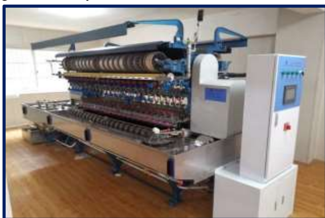
Figure 4. Modern automatic reeling machine capable of producing premium-quality raw silk with reduced labour requirements
