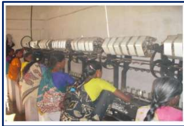
Figure 2. Cottage basin reeling unit—an improved system with separate cooking and reeling basins for better silk quality.
