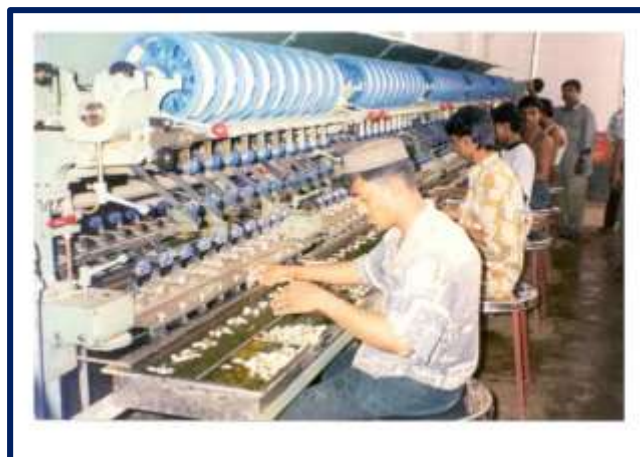
Figure 3. Multi-end reeling machine featuring croissure wheels, jetteboute, and planetary traverse for higher productivity and uniform yarn.
