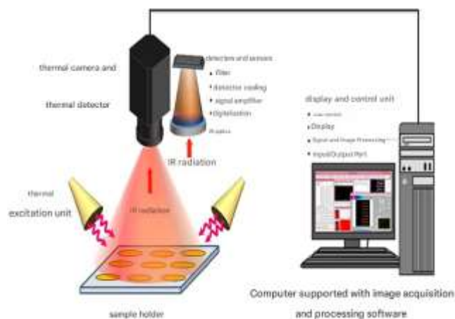
Figure 3: Thermal imaging setup (Source: Elmasry et al., (2020)).
